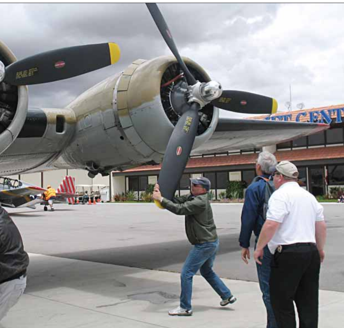
...ne times to ensure that excess oil from each of the nine pistons is removed. Below, l-r: The Witchcraft flew 130 missions under nose and tail gunners as well as bombardiers and ball turrets; swastikas on the B-17 bomber represent the number of destroyed
