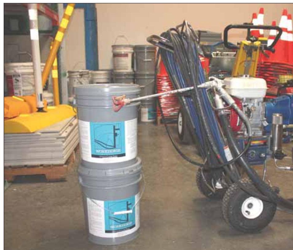
An airless spray rig is the tool workers at the city's operations services center use to cover up taggings. The rig uses reclaimed paint, shown above with the rig, which costs $35 for five gallons as opposed to $130 for new paint.
