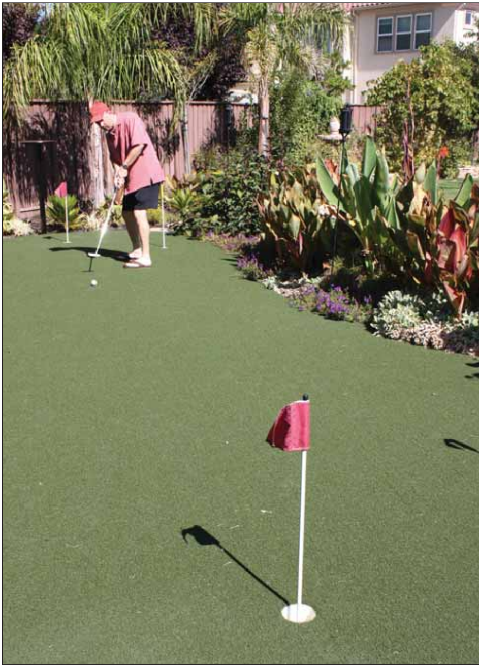
To perfect his putting green, Eric Steuben rolled down artificial grass with carpet glue and ordered the putting holes and flags online. The green rests on a concrete slab that peaks in the center, creating more angles and a higher level of difficulty for putting.
